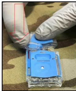
Figure A5. Sealing the cartridge
