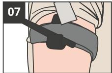
**ROUTE** the self-adhering band between the clips and around the rod
