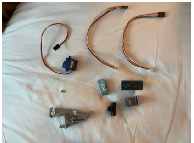
Sensor cables, servo, servo mount, and sensors
