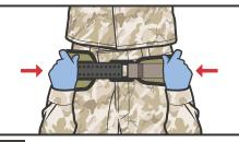
**MAINTAIN** tension and 07 immediately press free end of the strap onto the surface of the PCD. NOTE: Do not be concerned if you hear a second click after the PCD is secured.
